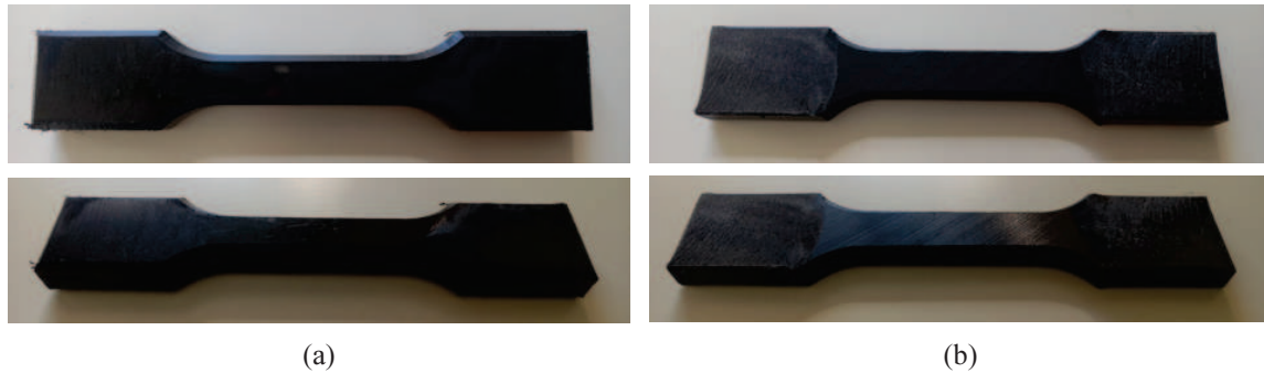
Figure 4. Dog-bone tensile test specimens: (a) virgin HDPE; (b) recycled HDPE.
