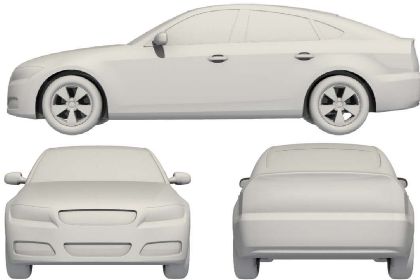
Figure 5.1: DrivAer in fastback configuration: on top - side view; on bottom from left to right - front and back views.
