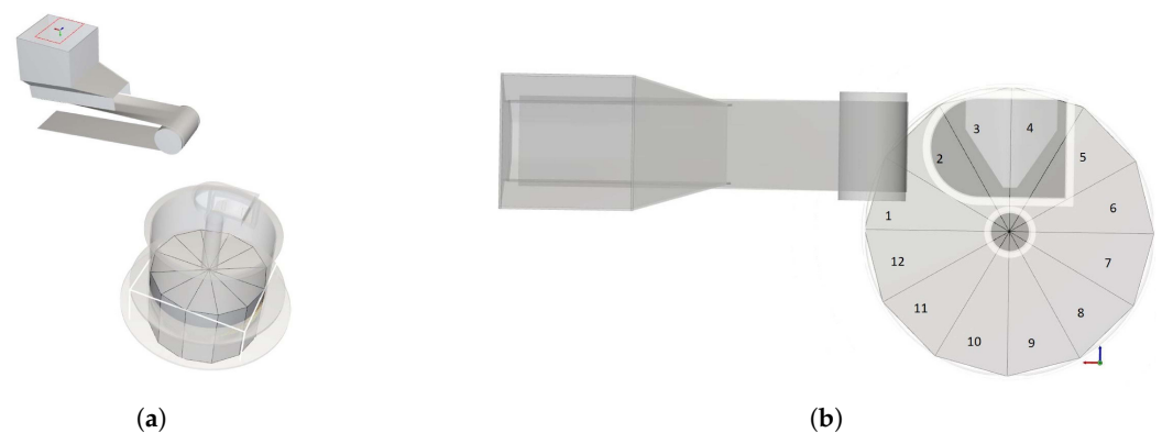
Figure 3. The radial sectors into which the hopper is ideally divided: (a) axonometric view; (b) top view with the numbering of the radial sectors into which the hopper is virtually split.
