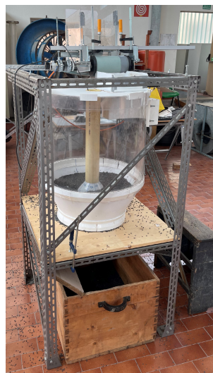
Figure 18. Laboratory-scale model of the system composed of the BF hopper, the conveyor belt, and the deflector used for experimental validation.
