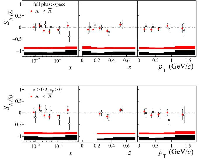
Fig. 4. Spin transfer  $S_{\Lambda(\bar{\Lambda})}$  for the full phase-space (top) and for the current fragmentation region (bottom), as a function of  $x$ ,  $z$  and  $p_T$ . The bands show the systematic uncertainties, while the error bars represent statistical uncertainties. The values in  $x$ ,  $z$  and  $p_T$  are staggered for clarity.
