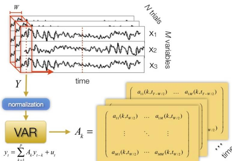
**Figure S1.** Explanation of the process for the calculation of the MVAR coefficients. The illustration on the top represents the EEG raw data of  $M$  variable,  $T$  time points, and  $N$  trials.  $W$  is the length of the sliding window that starts at the first time point of the signal, and steps until the end by a number of time points defined by the user.
