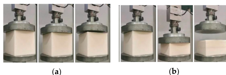
Figure 9. Compression-cycle press/hold/release; (a) 10% deformation, (b) 50% deformation.
