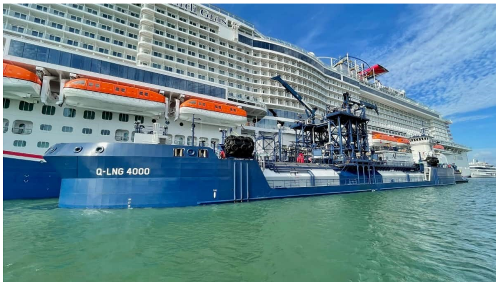
Figure 76 - Refuelling operations at LNG fuelled Carnival Mardi Gras [126]
