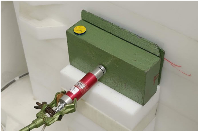
Fig. 4. Integrated CLYC detector placed at the output window of the DD generator, separated by a lead block to maximize the Cs-137 \gamma counts for calibration.
