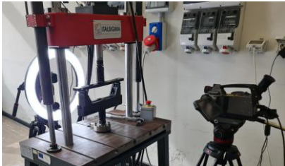
Figure 2. Experimental set up for bending tests.
