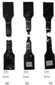
Figure 20. Some specimens of different typologies fractured during the tensile tests: (a) VT15BWE_5, (b) VT15BWM_6, (c) VT10BWM_1.
