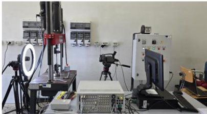
Figure 1. Experimental set up for tensile tests.
