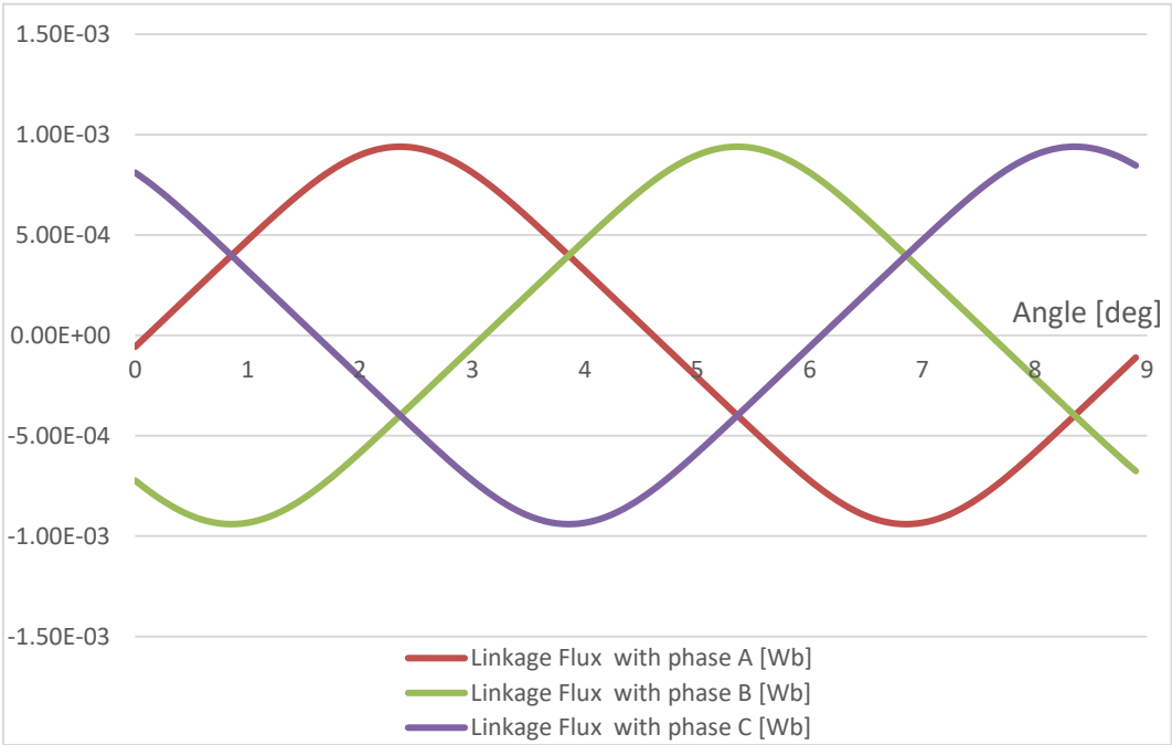
Figure 11: The flux linkages along a polar pitch with 2000A of model current.
