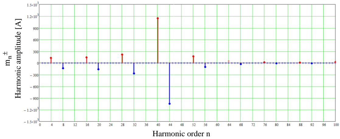
Figure 75: SPM machine MMF spectrum for the traditional star slot winding.
