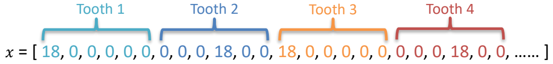
Figure 74: The x vector used for the winding optimization with the Fractional-slot concentrated algorithm.
