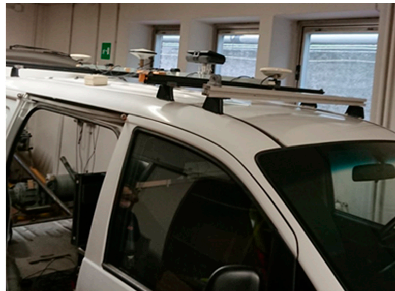
Figure 2. The setup of GNSS antennas, u-bloxes and smartphone on the roof of the vehicle.
