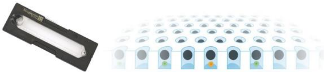
Figure 10: Microfluidic platforms for loading single cells. The figure illustrates a dedicated microfluidic platform (left) used for the controlled loading of single cells into individual wells (right). The use of these microfluidic systems ensures precise positioning of single cells.
