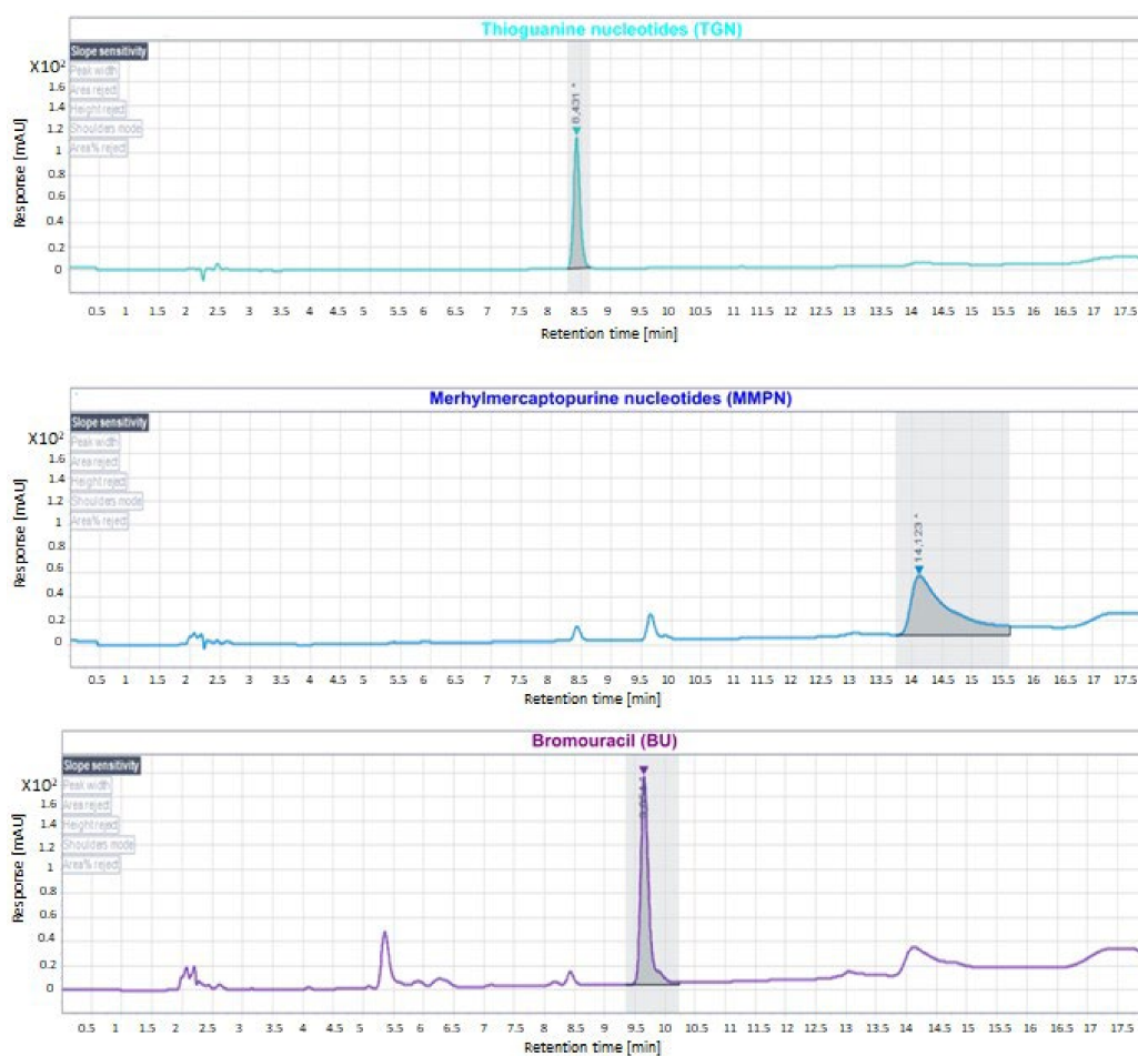
Figure 2. Chromatogram showing the retention times in minutes of the analytes TGN and MMPN (green and blue lines) and of IS (purple line). * indicates the retention times.
