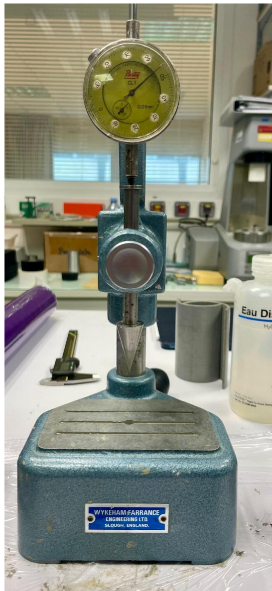
Fig. 2.17: Fall cone test equipment.
