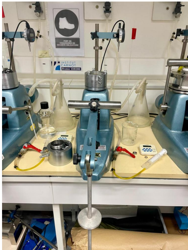
Fig. 2.13 Oedometer used for the consolidation test.
