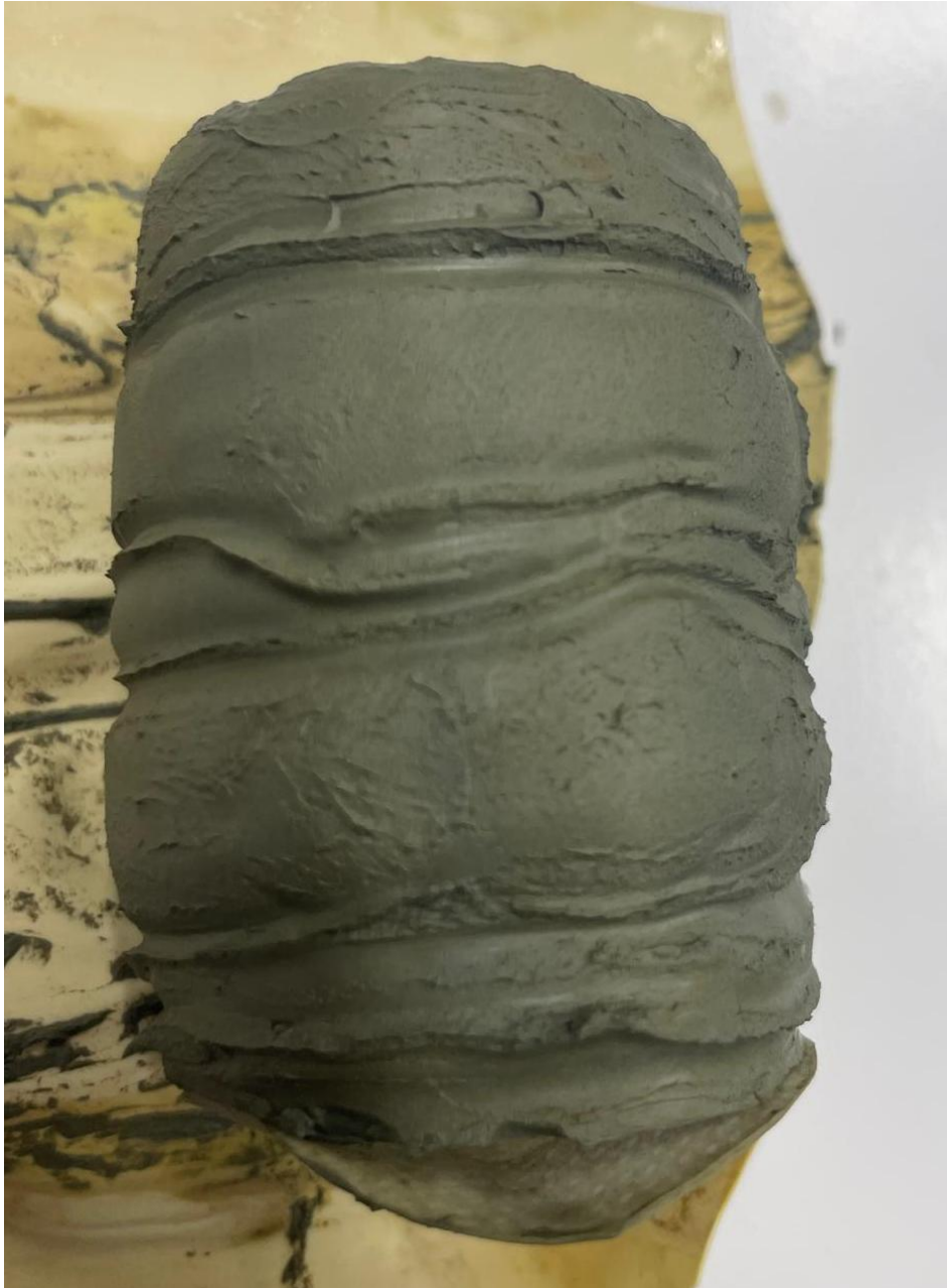
Fig. 2.16 Deformed sample after a triaxial test. The yellow background is the membrane that needs to be removed at the end of the test.
