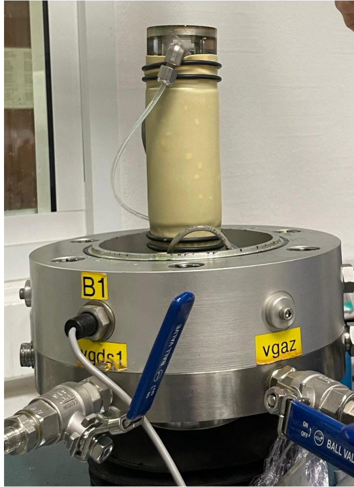
Fig. 2.14 Prepared specimen ready for the initial stage of the triaxial test.
