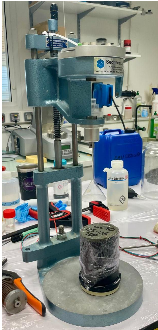
Fig. 2.12 Equipment used for the shear vane test.
