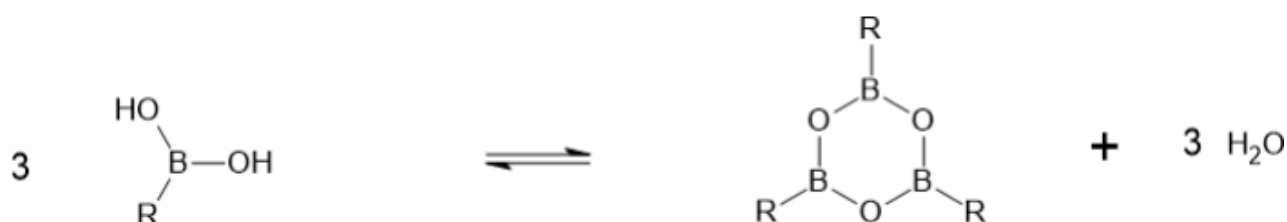
Figure 1.1 | Scheme of the condensation reaction of boronic acids into boroxines.
