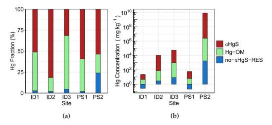
**Figure 4.** (a) Average relative abundance of  $\alpha$ -HgS, Hg bound to OM and residual no- $\alpha$ -HgS after oxidation; (b) average Hg concentrations in the various fractions.
