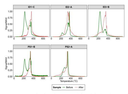
**Figure 5.** Comparison of Hg thermo-desorption curves before and after the oxidation test. The sample with the highest initial THg content for each site is shown.
