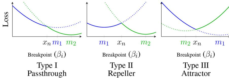
**FIGURE 3 |** Classification of critical points:  $p_1(\beta_i)$  shown in blue,  $p_2(\beta_i)$  shown in green; solid lines represent the 1 dimensional loss slice  $\tilde{\ell}(\beta_i; \beta_{-i}, \mu, s)$ , dotted lines represent the extension of  $p_k(\beta_i)$  past  $x_n$ .
