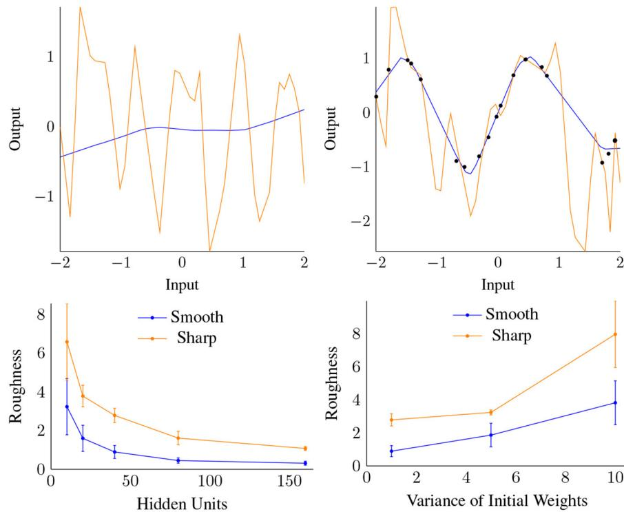
**FIGURE 10 |** Top: “Spiky” (orange) and standard initialization (blue), compared before (left) and after (right) training. Note both cases reached similar, very low training set error. Bottom: Roughness vs. Width (left) and the variance of the initialization (right) for both data gap cases shown in **Figure 11**. Each datapoint is the result of averaging over 4 trials trained to convergence.
