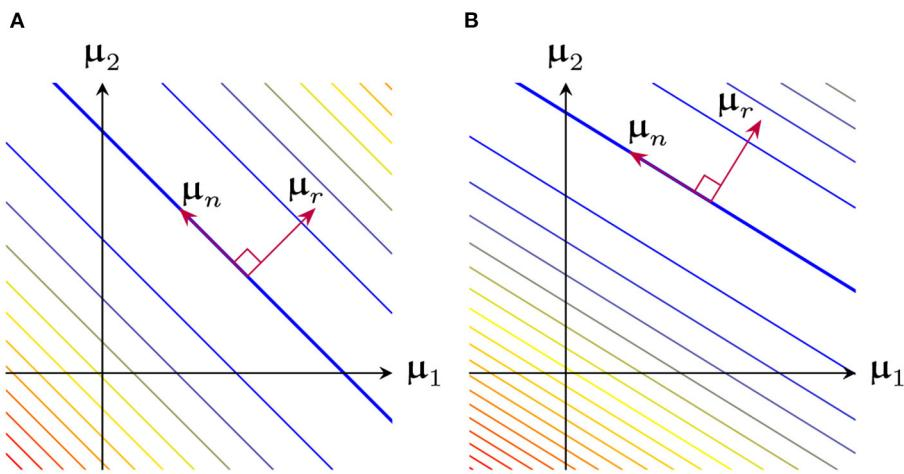
**FIGURE 6 |** 2-dimensional representation of the loss surface as a function of  $\mu$ , broken down into a loss-sensitive range and loss-independent nullspace **(A)** Example for fixed  $\beta$  **(B)** Same system as before, except  $\beta$  was varied, resulting in modified  $\mu$  range and nullspace.
