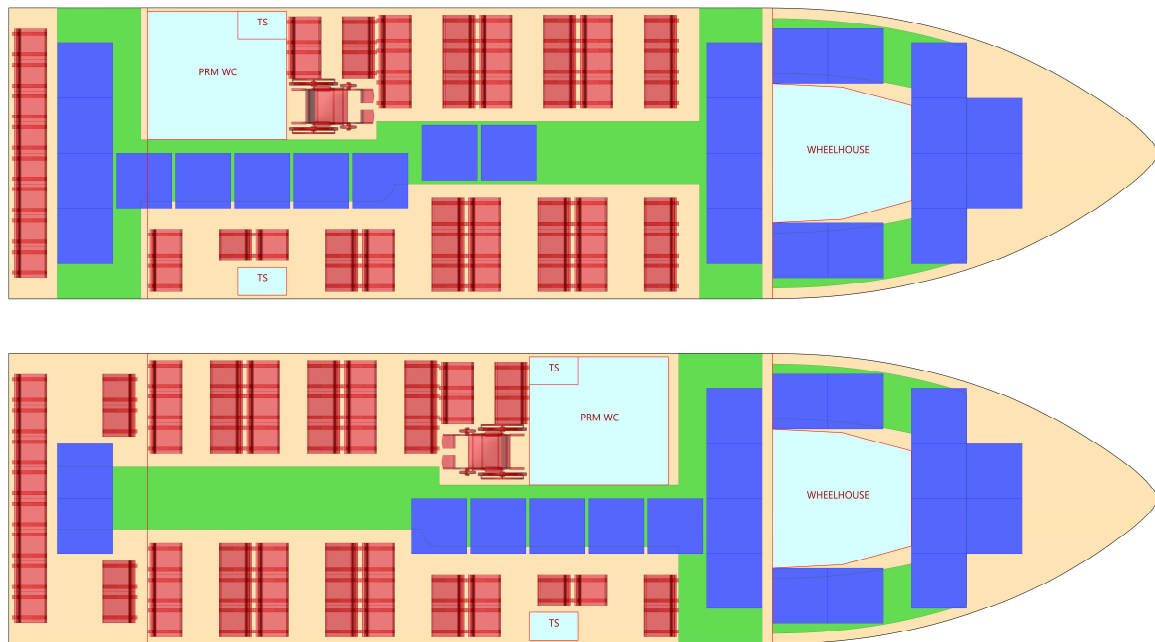
Figure 51 Influence of the longitudinal position of the PMR-compliant toilet compartment on the placement of the associated reserved seating within the passenger area. Seating in red, standing areas in blue, circulation corridors in green, technical/service spaces in light blue
