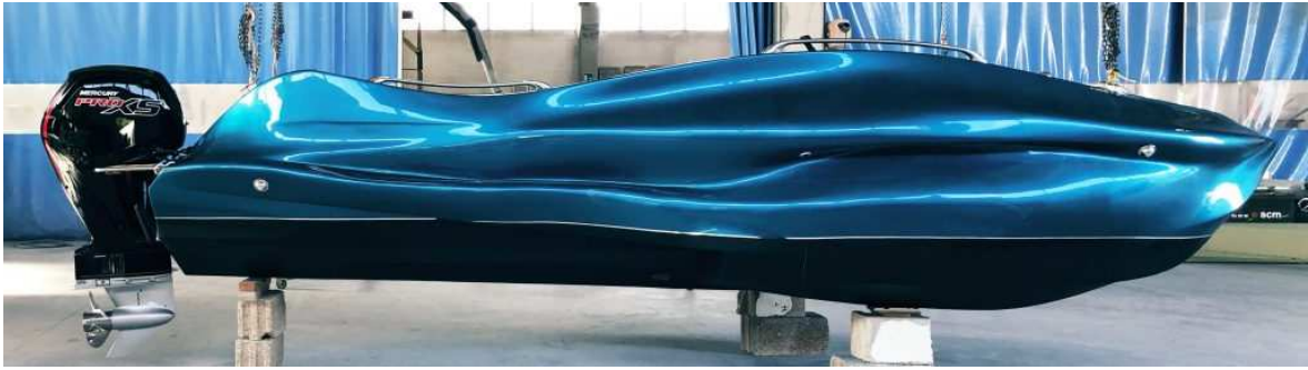
Figure 14 MAMBO prototype: an experimental GRP hull [ https://alumni.polimi.it/2020/10/14/la-prima-barca-al-mondo-in-fibra-di-vetro-stampata-in-3d-e-made-in-polimi/ ]
