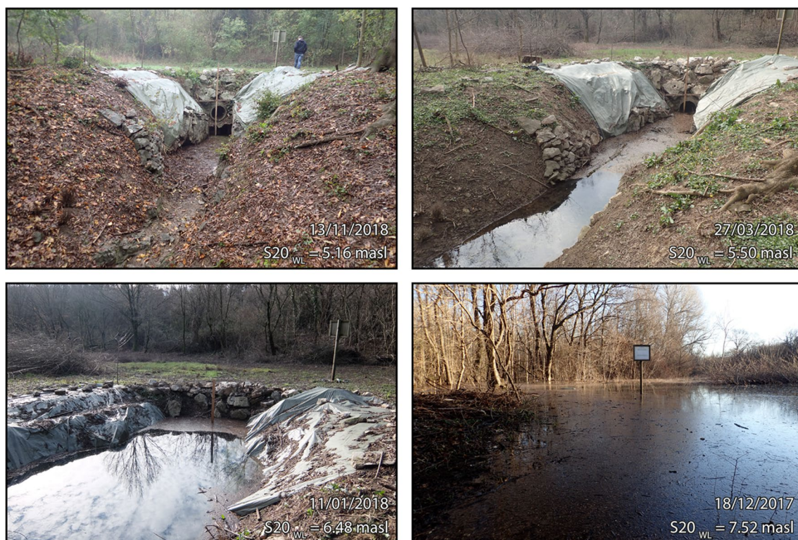
Fig. 2 Sw-02 swallow hole is the southernmost one in the study area. The discharge pipe is visible in the photo, taken on 13th November 2018 and 27th March 2018. The photographs illustrate the situation
