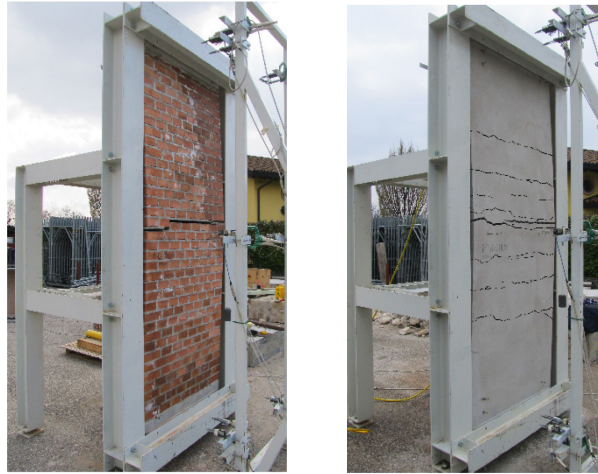
Fig. 2. Out-of-plane bending tests: damage pattern of (a) plain and (b) CRM strengthened masonry.
