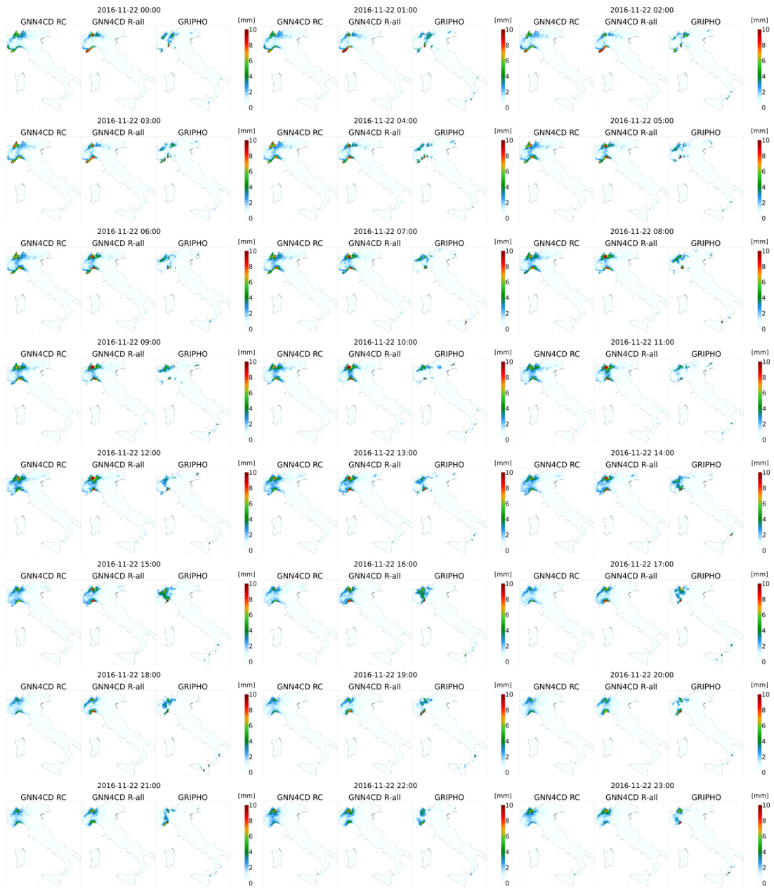
Figure 10.9: Reanalysis to observation downscaling: snapshots of precipitation [mm/h] for the first day of flood episode (1) in Figure 10.8 (22 November 2016).
