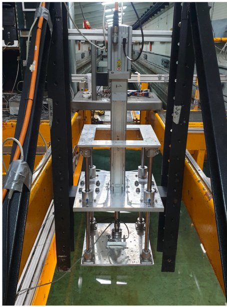
Fig. 3. Picture of the developed system (left). The actuator is attached to the system through a single DoF load cell. Parts of the developed system (right).
