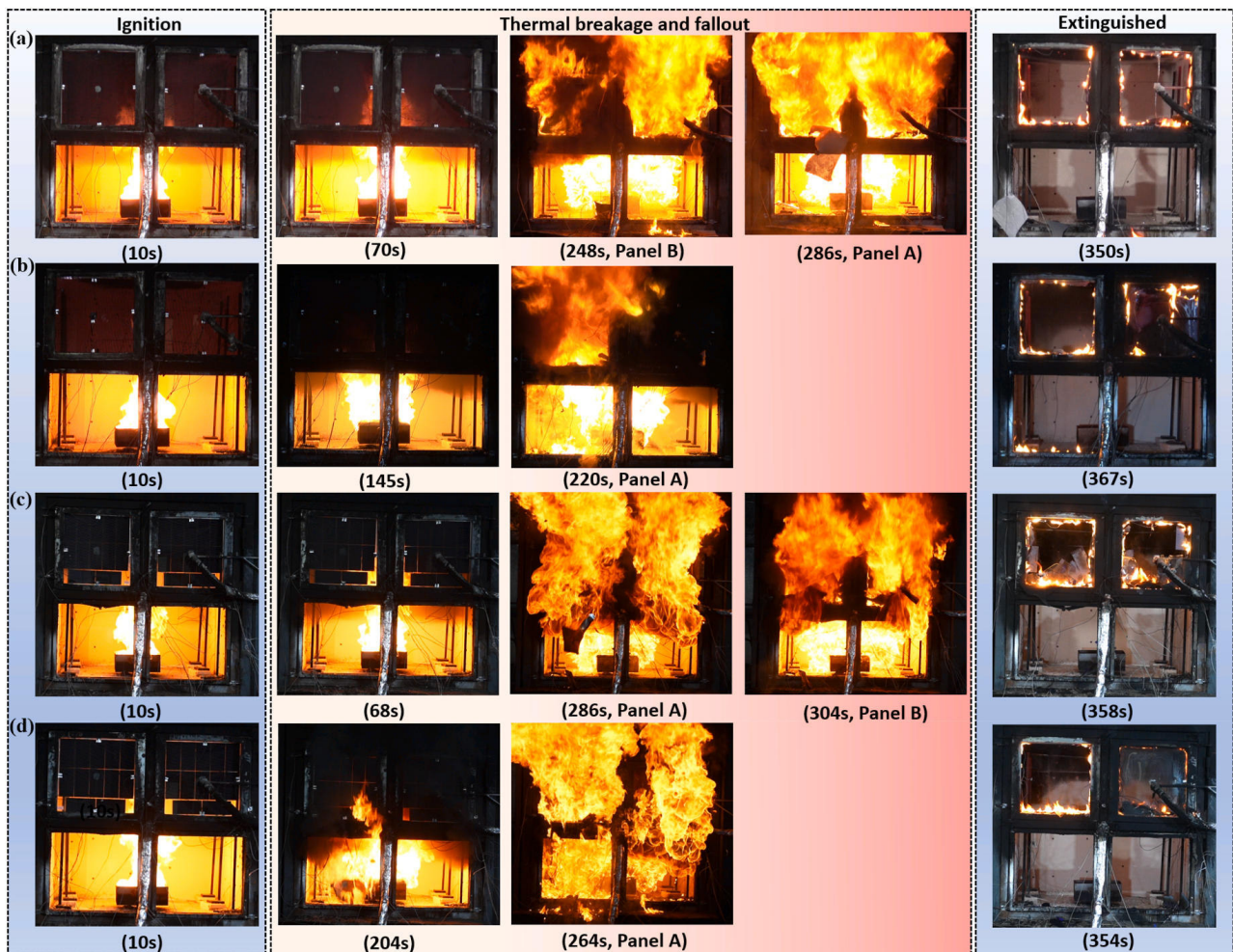
Fig. 5. Fire behavior of double-glazed PV modules. (a) Test 2 (Case 1); (b) Test 2 (Case 2); (c) Test 2 (Case 3); (d) Test 2 (Case 4).
