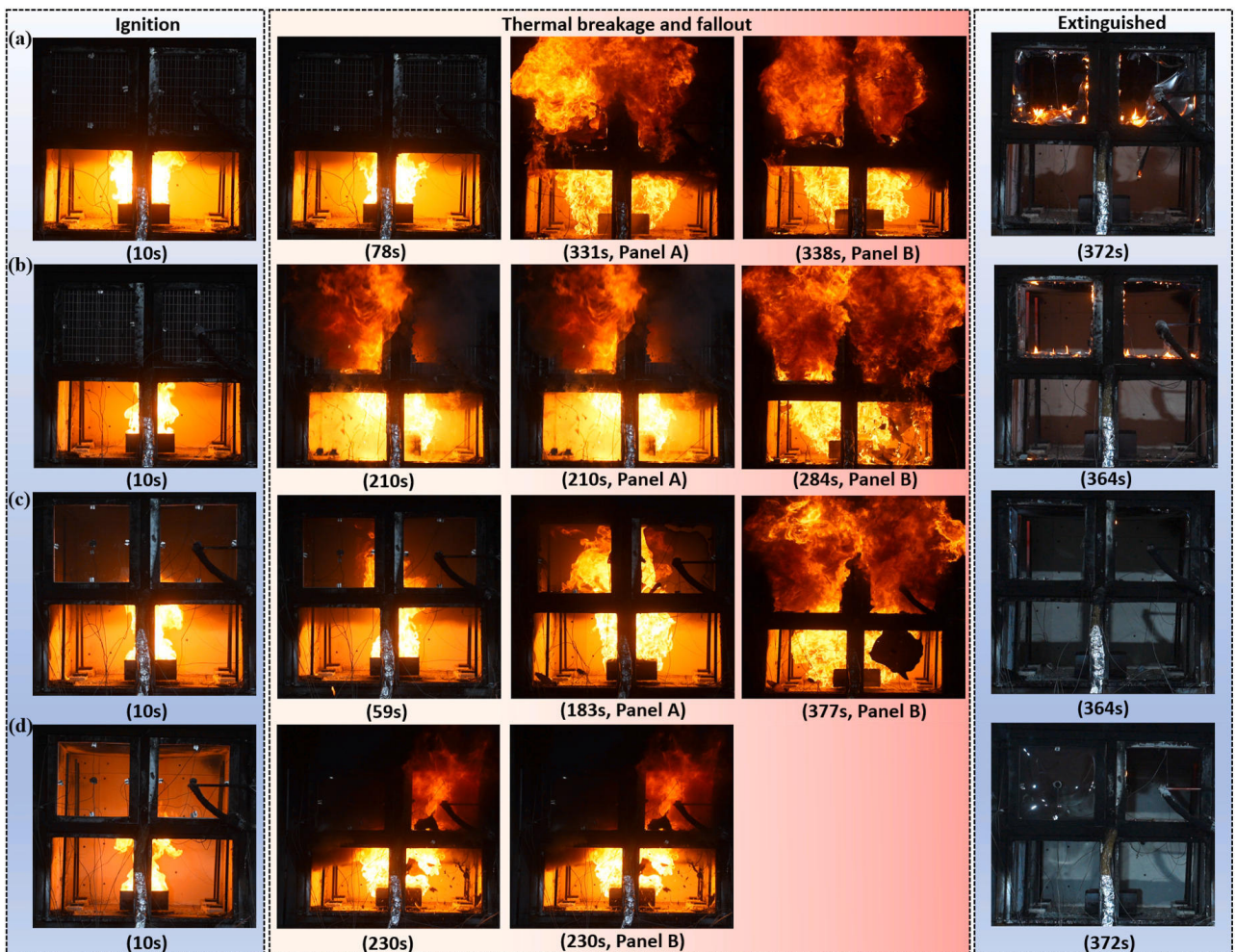
Fig. 7. Fire behavior of single-glass PV modules. (a) Test 1 (Case 5); (b) Test 2 (Case 6); (c) Test 1 (Case 7); (d) Test 1 (Case 8).
