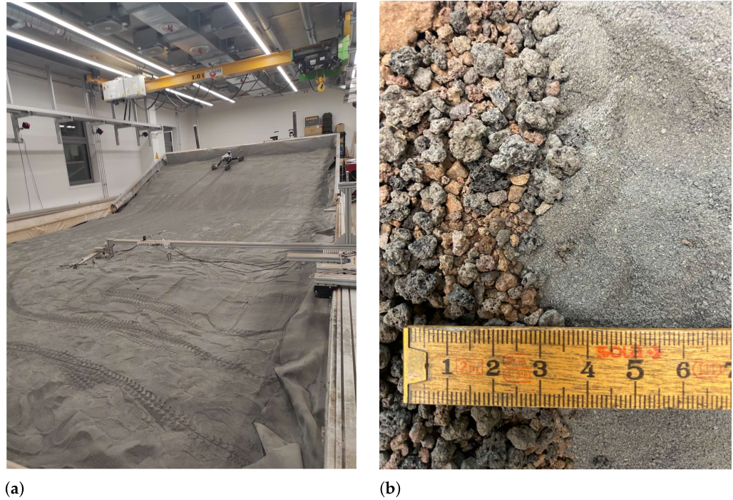
Figure 7. Experimental setup. (a) The DLR PEL sandbox and the rover climbing a 20° slope. (b) The two types of soil, shown side by side.
