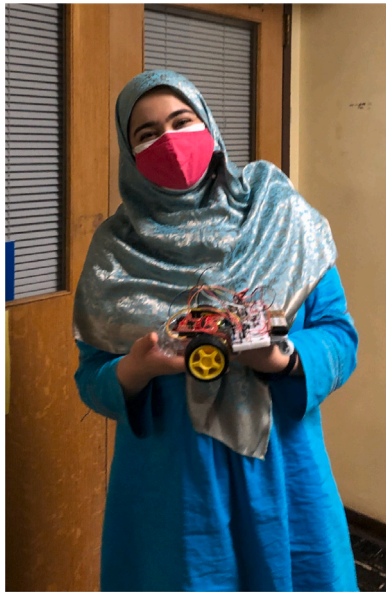
Fig. 1. A proud student showing off her final project, the voice-controlled robot car in EECS16B at UC Berkeley at the end of her first year. The project uses principal-components-analysis to learn the voice commands and pole-placement for control of the car.
