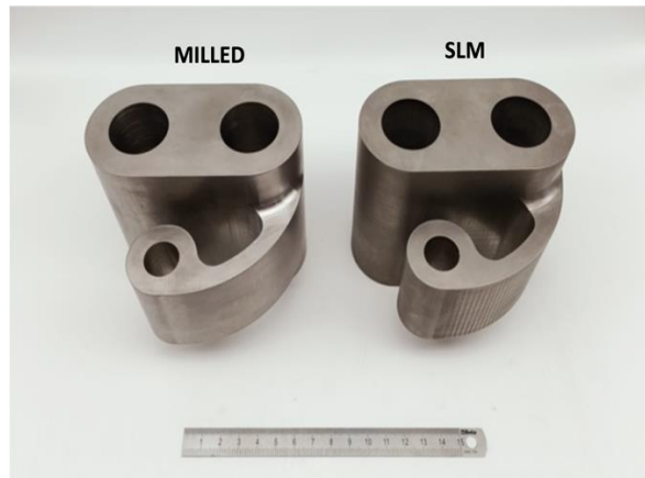
Fig. 6. Milled and SLM wishbone mock-up of the DEMO diverting device.
