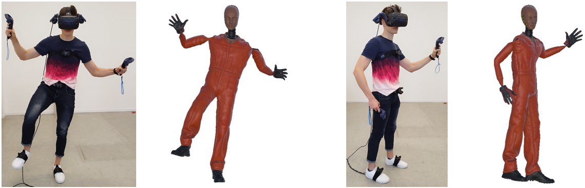
Figure 4.74: Adaptation of the virtual body to the real-time movement ([83]).
