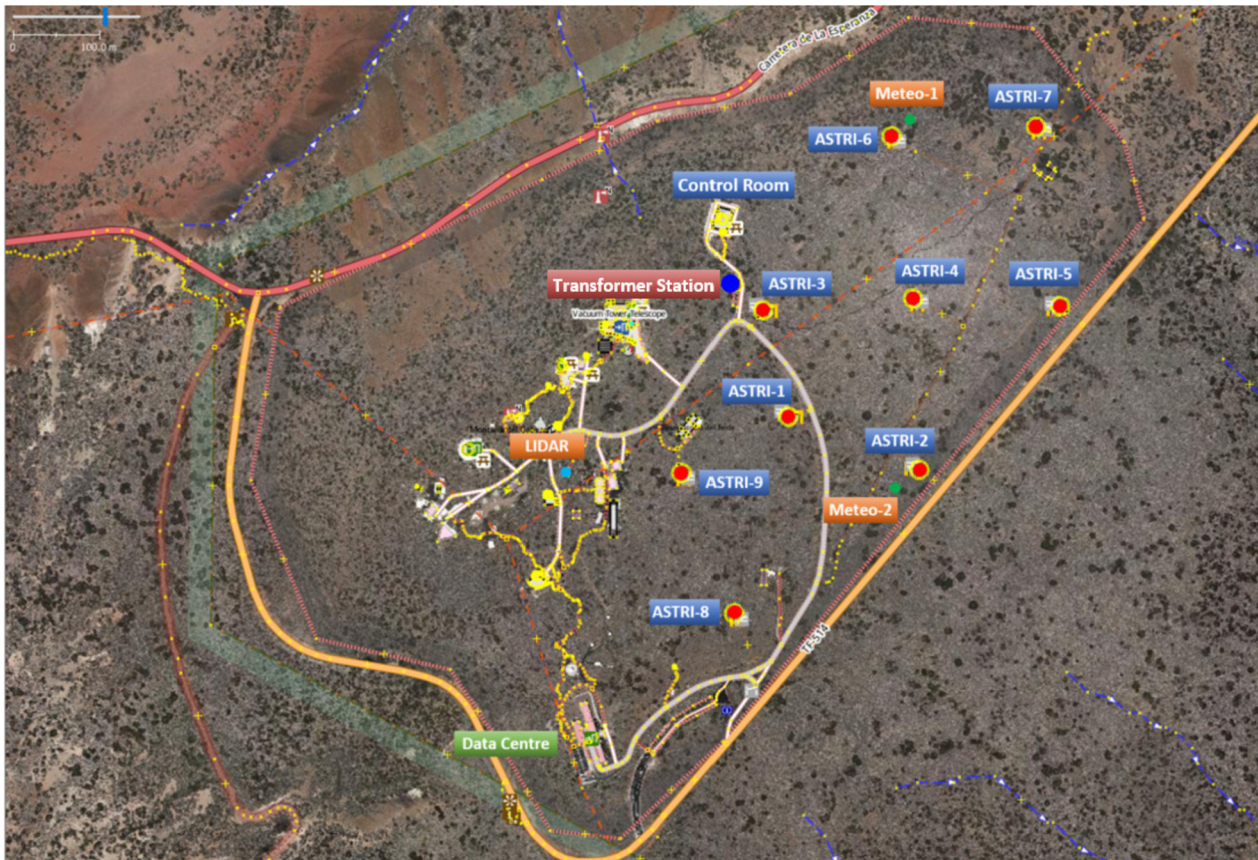
Fig. 2. The final layout for the ASTRI mini-array. The Figure shows the final positions for the 9 telescopes, the position of the two meteorological towers, the position of the LIDAR, the position of the transformer station and that of the local control room and of the data centre. (Image obtained with Open Street Map editor).
