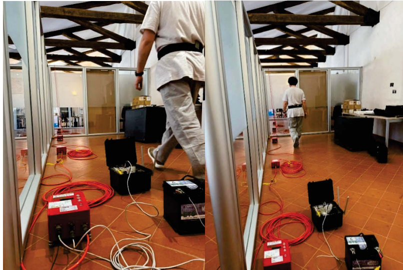
Fig. 118 – Walking tests in the historical palace.
