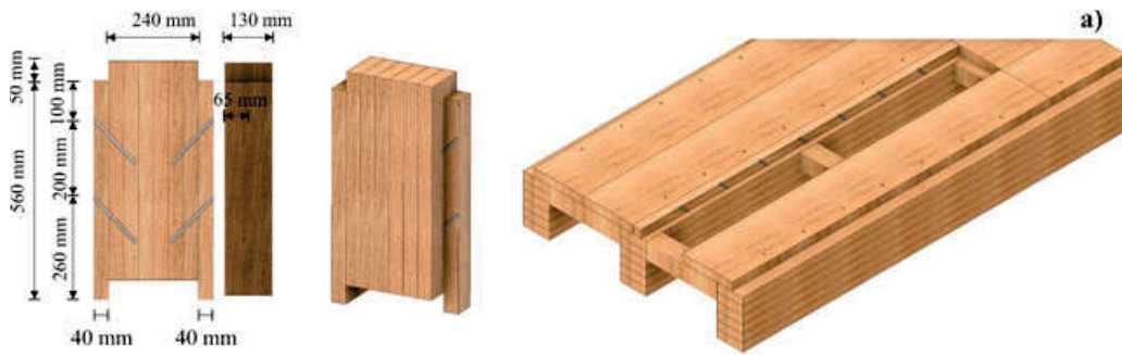
Fig. 49 – Pushout test geometrical configuration.
