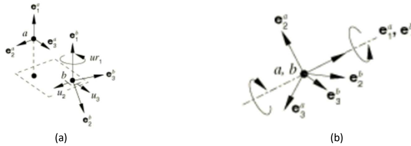
Figure A.4-6 Planar connector type for glass-frame connection; and (b) hinge connector type for transom-mullion connection (Abaqus library)
