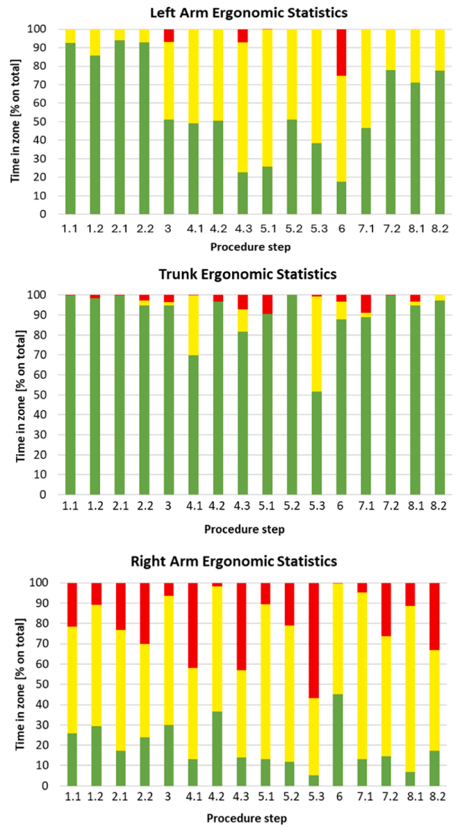
Fig. 16. Ergonomics results of the maintenance procedure: Left arm (top), trunk (middle) and Right arm (bottom).
