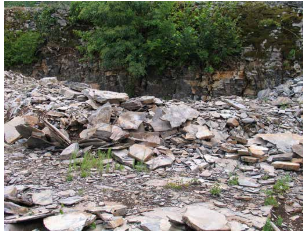
Figure 5.1.6: Abandoned surface extraction of the Komen platy limestone in Gabrovica (Slovenia), used for roofing and paving (Photo: Bogdan Jurkovšek)
