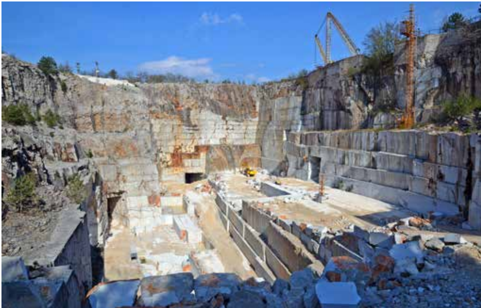
Figure 4.2.11: The Lipica 1 Quarry lies northeast of the well-known Lipica Stud Farm. In this quarry, large blocks of massive Cretaceous limestone are exploited. The quarry is situated in the most economically promising part of the Lipica Limestone in the north wing of the Lipica syncline, a large bowl-shaped fold with an axis slightly plunging towards the southeast (Photo: Matevž Novak)
