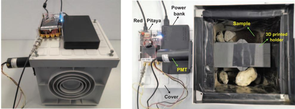
Fig. 1. – Left: the box with the detector inside, the *Red Pitaya STEMLab 125-14* and the power bank (20000 mA/h) on the top. Right: the inner part of the box. From left to right: the *Red Pitaya STEMLab 125-14* and the power bank placed on the lid of the box that contains the environmental sample and the 3D case with the photomultiplier tube and the CsI:Tl crystal.
