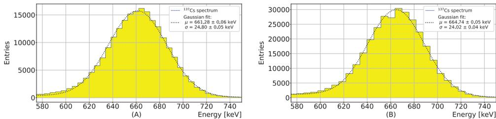
Fig. 2. – 662 keV photoelectric peak of a  $^{137}\text{Cs}$  source, acquired with a Saint Gobain NaI:Tl, used to measure the energy resolution with the portable system (A) and with the standard one (B).
