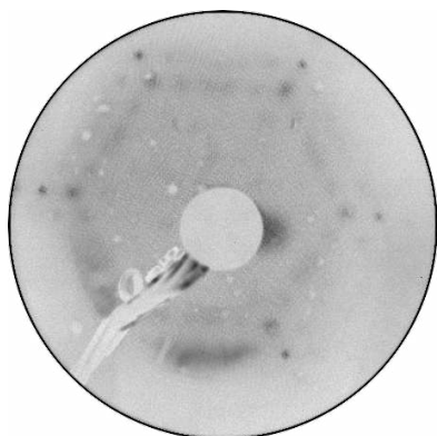
(c) LEED diffraction pattern of BlueP/Au(111) at E=60.6 eV ( \theta \sim 0.8 ML)
