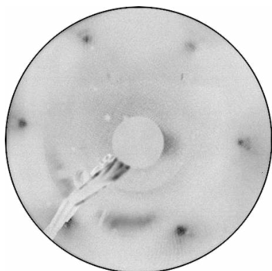
(a) LEED diffraction pattern of clean Au(111) surface at E=60.6 eV
