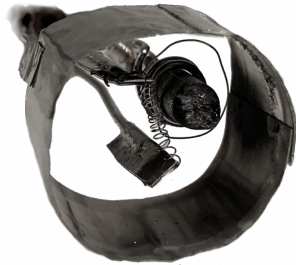
Figure 3.1: Homemade evaporator, exploiting electron bombardment of a solid B rod from a tungsten filament, limited by a Wehnelt and isolated by a Tantalum screen.
