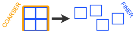
Figure 3.9: Sketch representing the impact of decreasing grid spacing on the number and positions of updraft cores with the convective fraction \epsilon being kept fixed.
