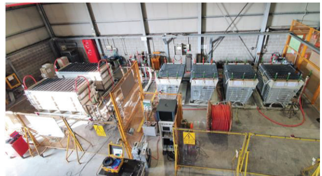
Figure 4 – Overall view of the second experimental set-up reproducing humid and rainy periods.
