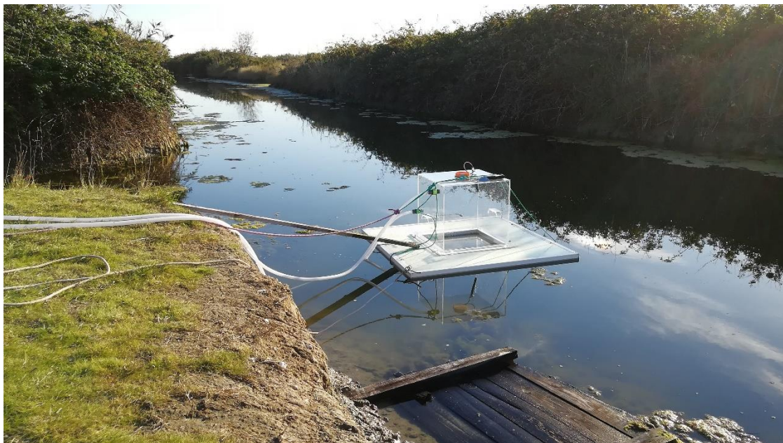
Figure 12: the floating flux chamber during a measurement at site VN.
