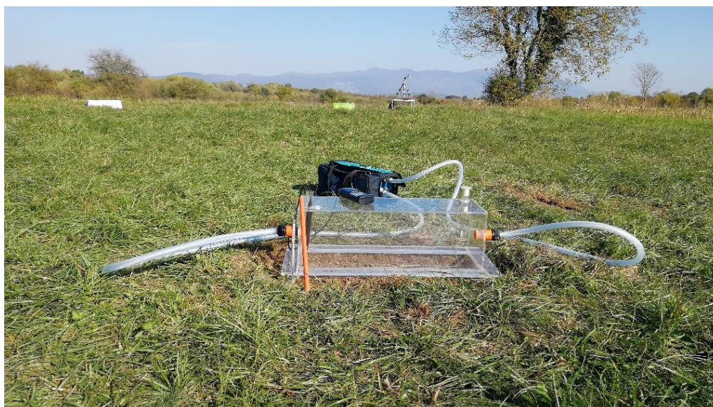
Figure 13: the NSS flux chamber during a measurement at site SAV.
