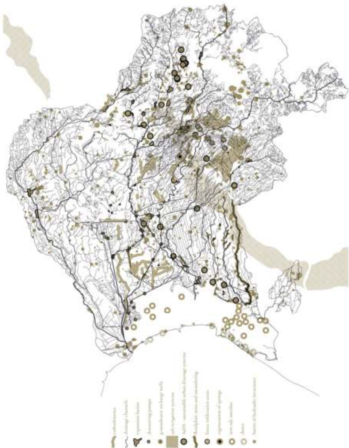
Synoptic representation of the adaptation works of the hydrographic system for the drainage basin of the Venice lagoon.
