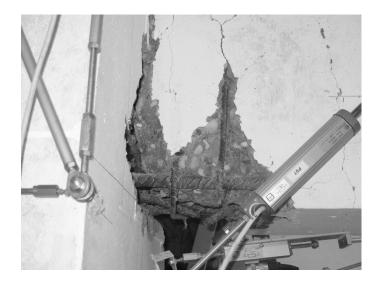
Fig. 12. Tensile break of a beam bottom bar during the 70 mm step for specimen J2.
