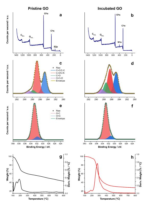
**Fig. S4** Survey spectra for pristine (a) and incubated (b) GO. Deconvoluted high resolution spectra of C1s and O1s core levels for pristine (c, e) and incubated (d, f) GO. TGA weight loss and first derivative curves under inert conditions of pristine (g) and incubated (h) GO.
