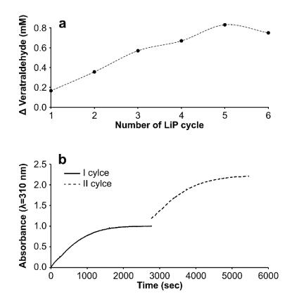
**Fig. S1** Variation of veratraldehyde after the consecutive activation of 6 LiP catalytic cycles in the same blank sample (a). Veratraldehyde production in two consecutive LiP catalytic cycle (b). Blank samples are made of 30  $\mu$ L of 150  $\mu$ g mL<sup>-1</sup> LiP suspension, 5.6  $\mu$ L of 1.5 M veratryl alcohol, 0.4  $\mu$ L of 0.21 M H<sub>2</sub>O<sub>2</sub> and 964  $\mu$ L of tartaric acid/sodium tartrate buffer solution.
