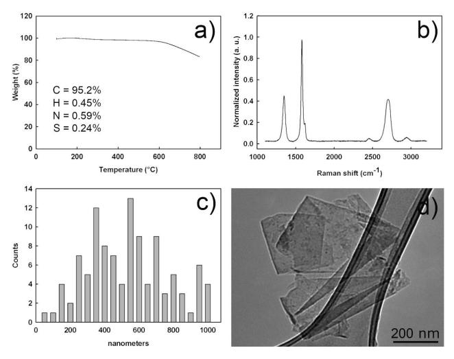
**Fig. S2** Physicochemical characterization of FLG: thermogravimetric and elemental analysis (a); average Raman spectra (b); lateral size distribution of the sheets (n = 100) (c); and representative TEM image of FLG (d).
