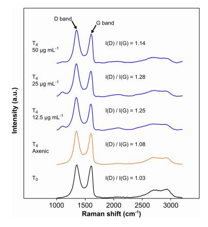
**Fig. S3** Average Raman spectra of untreated GO flakes ( $T_0$ ) and of GO flakes incubated for 4 months ( $T_4$ ) in axenic culture media or in *P. chrysosporium* cultures at GO concentrations of 12.5, 25, and 50  $\mu$ g mL<sup>-1</sup>.
