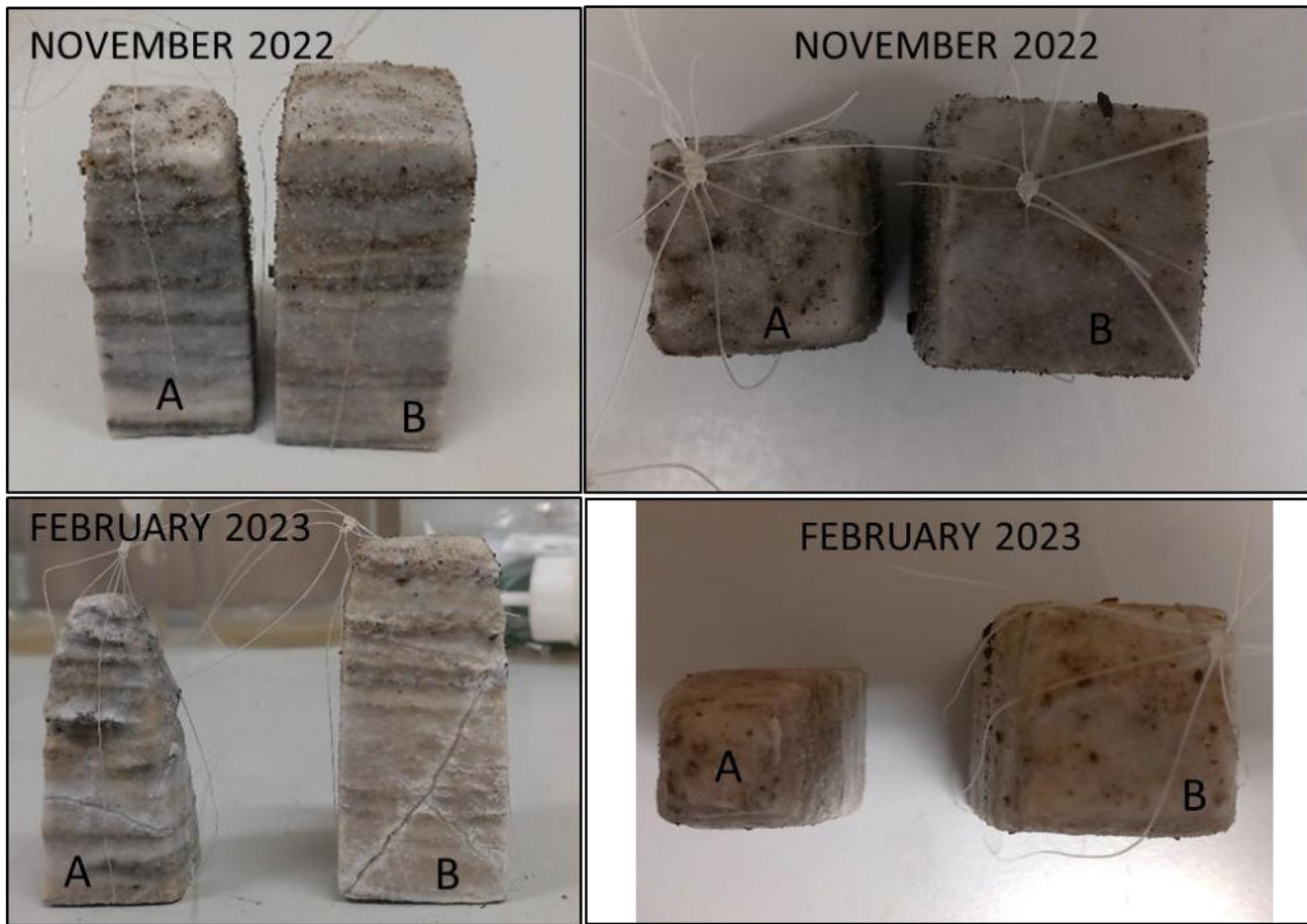
Figure 41 Comparison of rock samples between November 2022 and February 2023. Sample with daily changing water is marked with letter A, and sample with weekly changing water marked is with letter B
