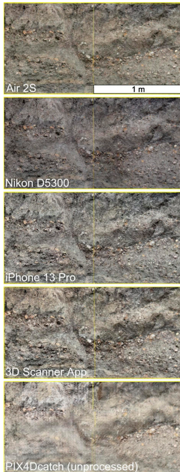
Figure 5. Detailed view of the reconstructed scene ( 2 \times 1 m) using different 3D image capture systems and showing one sidewall of the studied sinkhole.
