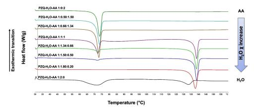
Figure 3. DSC results of the tests conducted in the presence of H<sub>2</sub>O-AA mixture.
