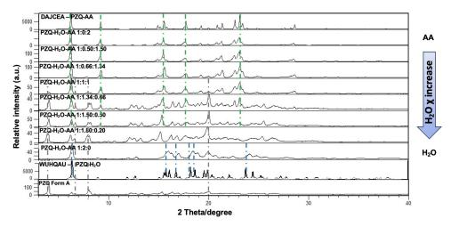
**Figure 2.** PXRD results of the tests in the presence of H<sub>2</sub>O-AA mixture. Green, blue and grey dotted lines highlight PZQ-AA, PZQ-HH and PZQ reflections, respectively.
