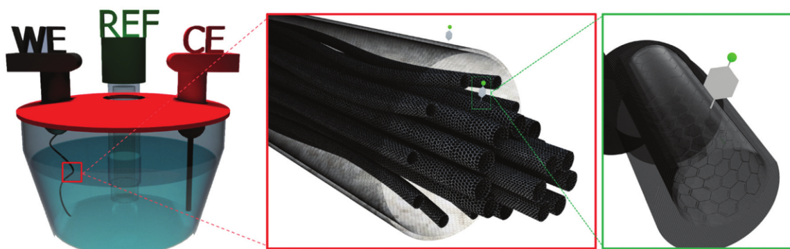
Fig. 1 Modified CNTFs with p -substituted phenyl ring through electrochemical reduction of aryl diazonium salt. Green ball corresponds to a general functional group.
