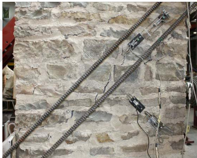
Fig.10. Diagonal crack in the URM specimen DC1.
