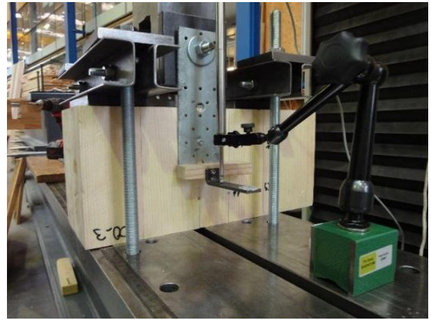
Figure 2. Experimental setups - (a) Tension tests, (b) bending tests, (c) nail withdrawal tests and (d) joint shear tests.
