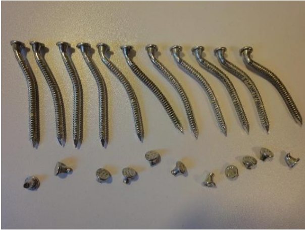
711 Figure 9. Single fastener joint shear tests - Deformed fasteners (a) after monotonic tests and (b) after cyclic tests.
