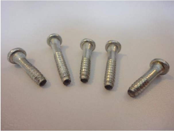
693 Figure 5. (a) Failure modes of the tension tests and (b) deformed fasteners after bending tests.
