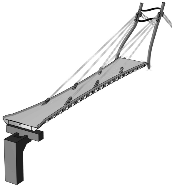
Fig. 10 Refined FE model M02 (ABAQUS/Standard). First vibration mode at 1.599 Hz.
