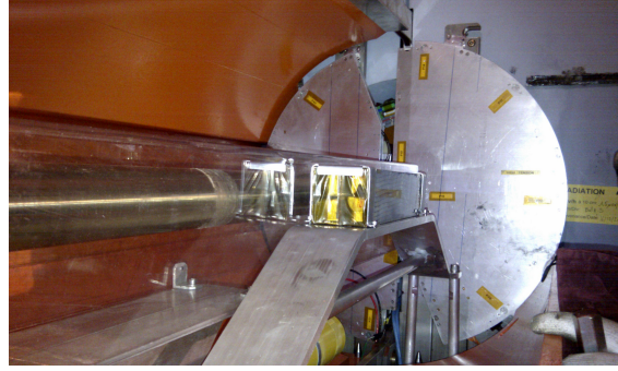
Figure 4. Schematic and photo of the 2 \times 2 EE-sized crystals irradiated close to the CMS beam pipe in 2012.
