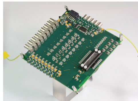
Figure 5: Front end electronics board with the plastic box enclosing the SDD.
