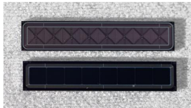
Figure 2: SDD linear array comprising 8 squared cells 3 \times 3 \text{ mm}^2 . Anode (top) and entrance window (bottom) sides.
