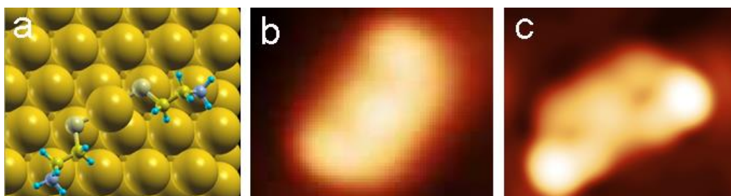
Figure 6.10: (a) stick and ball model for DFT-optimized “E” chiral complex and its relative (b) experimental and (c) simulated STM images.
