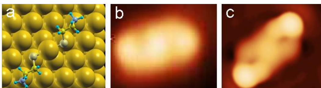
Figure 6.11: (a) stick and ball model for DFT-optimized “S” chiral complex and its relative (b) experimental and (c) simulated STM images.
