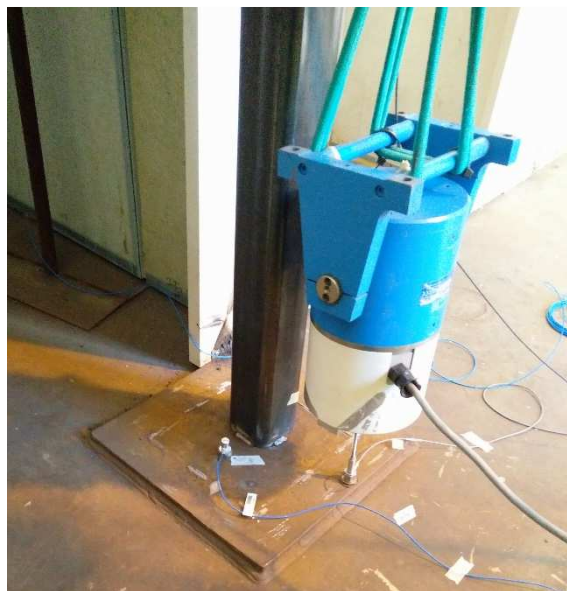
Figure 5.3 - Shaker connection near the base of the pillar
