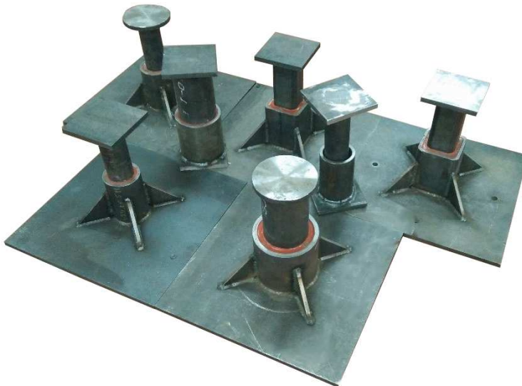
Figure 8.1 - Pillar isolator prototypes
