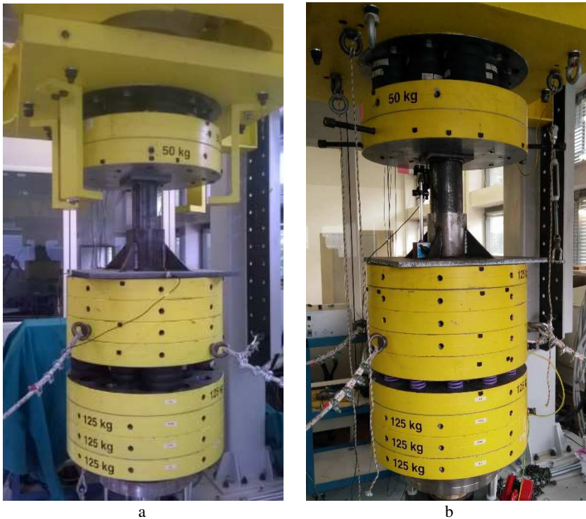
Figure 9.1 - High frequency test rig initial configuration (a) and improved configuration (b)
